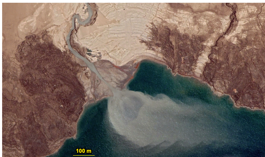
FIGURE 7 Buoyant plume of the Jordan River over the Dead Sea: Note that, because of the excess of buoyancy induced by the high \Delta\rho_b , part of the river momentum is transferred to the overflow, resulting in a narrow and elongated buoyant plume. Image from Google Earth, June 2019.
